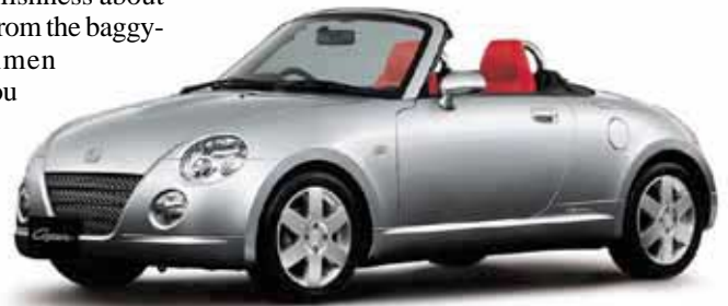
The Daihatsu 'Copen' turbo-charged .665 liter engine, 63 horsepower at 6,000 rpm, 43 miles per gallon, top speed, 106 mph, $13,000. Not for sale in the United States.
